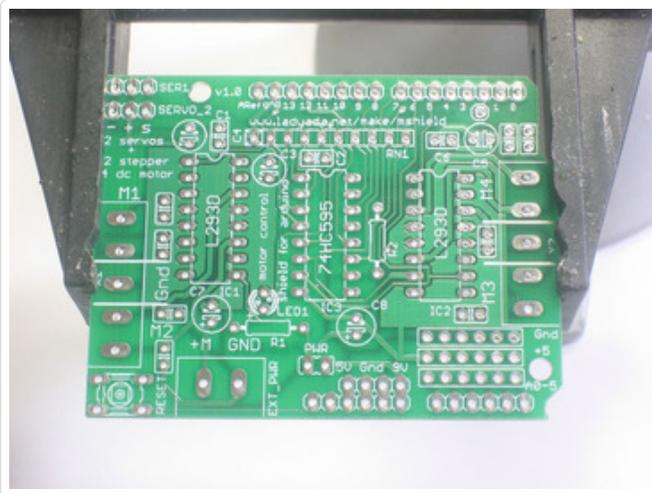
Place the motor shield PCB in a vise or other circuit-board holder and turn on your soldering iron to 700 degrees.
