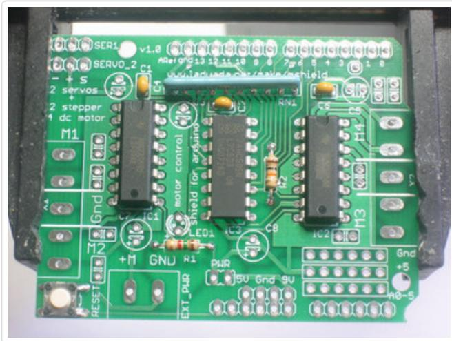
ICs must be placed in the correct orientation to work properly. To help with placement, each chip has a U notch at the top of the chip. On the circuit board there is a printed out image of the chip outline and one end has a U notch. Make sure the chip notch is on the same end as the image notch. In this PCB, all are facing the same way.
