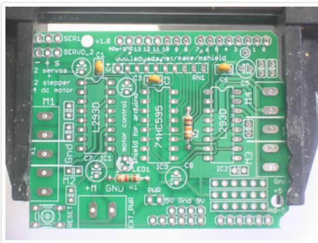
Next place the three yellow ceramic capacitors **C4**, **C2** and **C6**. Ceramic capacitors are not polarized so you can put them in "either way" and they work fine.
