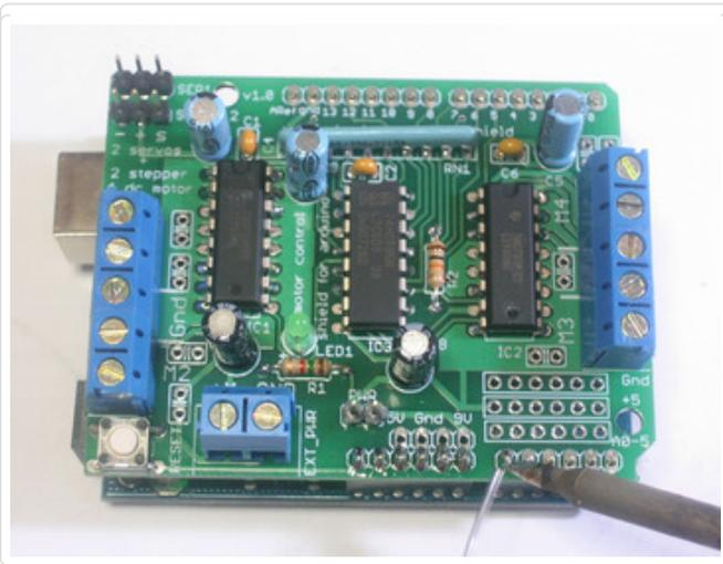
Solder in each pin of the header.
