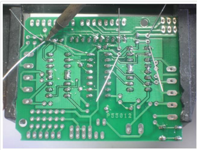
After double-checking their polarity, solder and clip the three capacitors.
