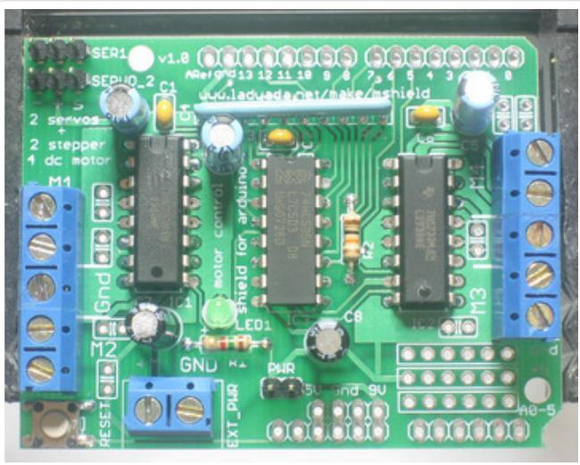
Solder in the 3 pieces of header and the three terminal blocks.
