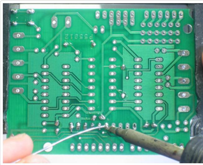
Flip the board over and solder in the resistor network and switch. You won't need to clip the leads as they are quite short already.
