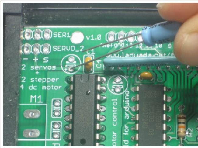
capacitors **C1**, **C3** and **C5**. Electrolytic capacitors are polarized and must be placed in the correct orientation or they could pop! The long leg of the capacitor is the positive (+) leg and goes into the hole marked with a +. The close-up images shown here indicate with hole is the + one.
