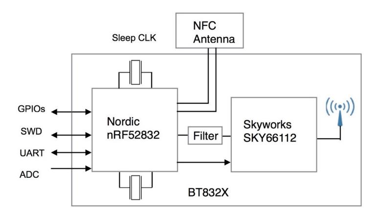
A high performance PCB trace antenna is integrated on BT832X. An u.FL connector on BT832XE provides connection to an external antenna. In this data sheets, both BT832X and BT832XE can be referred as BT832X.
