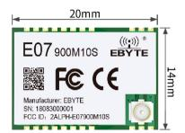
Since the module is a pure RF transceiver module, you need to use the MCU driver or a dedicated SPI debugging tool.
