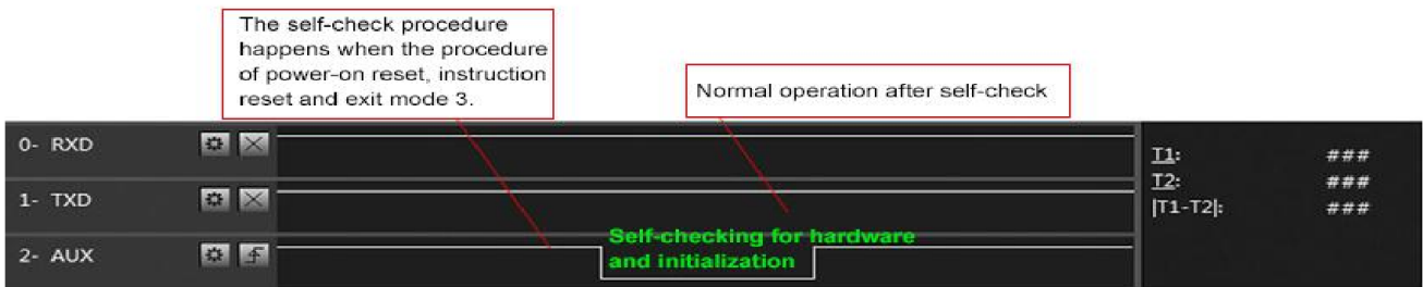
Timing Sequence Diagram of AUX when self-check
